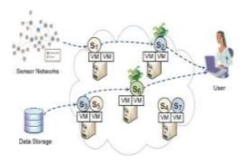
Fig. 1. Service integrity attack in cloud-based data processing. Si denotes different service component and VM denotes virtual machines
